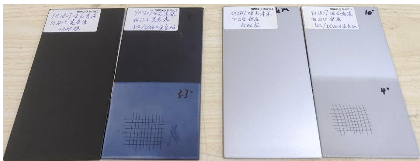
Alkali resistance (5%NaOH) 50°C immersion for 4h
